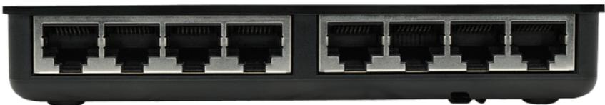
All ports on the Gigabit Ethernet Desktop Switch support Auto-MDI/MDI-X functionality, so crossover cables and uplink ports are not needed for connections to PCs, routers, hubs, additional switches or other devices. Cat5/5e UTP/STP cables provide optimal performance; if a top-panel LED corresponding to any of the ports in use doesn't indicate a link or activity, check the connected device for proper setup and operation.
